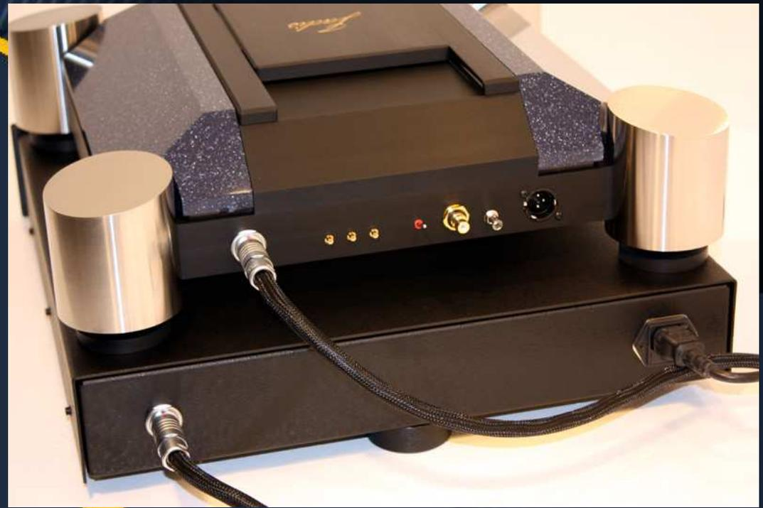
Based on Philips CDM12ProII mechanism, this new drive is equipped with the last and well known CD technologies. It also provide special digital signal on special connectors. These digital signal are specially designed to feed our future DSP controled DAC
