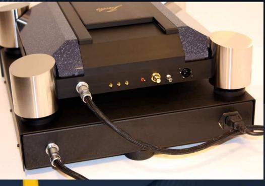
Based on Philips CDM12Proll mechanism, this new drive is equiped with the last and well known CD technologies. It also provide special digital signal on special connectors. These digital signal are specialy designed to feed our future DSP controled DAC
